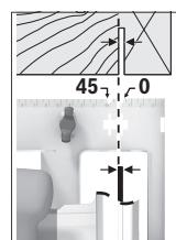
The 0° cut mark (9) indicates the position of the saw blade when making a right-angled cut. The 45° cut mark (8) indicates the position of the saw blade when making a 45° cut.
