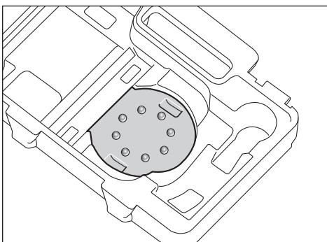
The alignment aid that is in the tool box and shown in the figure enables easy alignment of the sanding sheet (6) on the sanding pad (5). Place the sanding sheet into the alignment aid with the hook-and-loop fastening facing upwards and press the power tool with the sanding pad firmly onto it.
