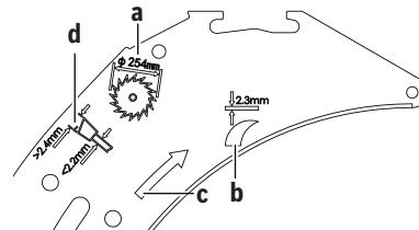
**a** The saw blade must be no more than 254 mm in diameter.
