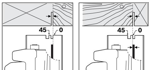
The 0° cutting mark (**8**) indicates the position of the saw blade for right-angled cuts. The 45° cutting mark (**7**) indicates the position of the saw blade for 45° cuts.
