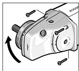
The machine head can be rotated with respect to the machine housing in 90° steps. In this manner, the On/Off switch can be brought into a more convenient position for special working situations, e.g., for cutting operations using the cutting guide with dust extraction protection guard 24 or for left-handed persons.
