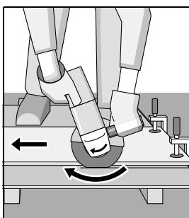
The machine must always work in an up-grinding motion. Otherwise, the danger exists of it being pushed **uncontrolled** out of the cut.
