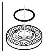
A plastic part (O-ring) is fitted around the centring collar of mounting flange 7. If the O-ring is missing or damaged, the mounting flange 7 must be replaced before resuming operation.
