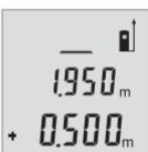
Press the button (6) to add measured values or press the button (3) to subtract measured values. "+" or "-" will appear at the bottom of the display. Take another measurement. The current measured value will be shown at the bottom of the display, and the previous measured value will be shown above it.
