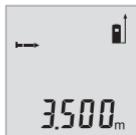
Move the measuring tool until the required distance is shown at the bottom of the display (1).
