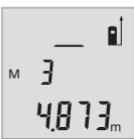
The number of the measured value is displayed after "M", and the respective measured value is displayed underneath.
