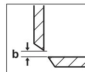
For adjustment of cutter clearance **b**, the stroke mechanism (7) of the upper cutter must be at the upper dead centre point. For this, briefly switch the power tool on and then immediately off again. If the stroke mechanism does not stop at the upper dead centre point, repeat the process.
