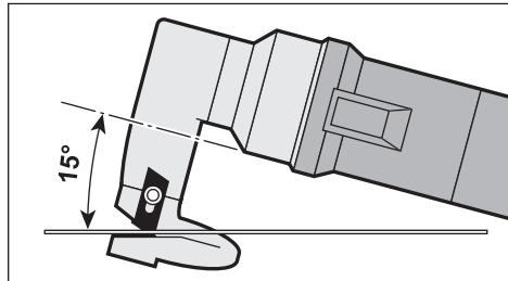
Hold the power tool inclined at an angle of 15° to the surface of the steel sheet and do not tilt it laterally.
