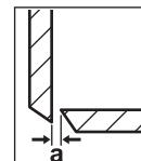
The cutter clearance **a** (gap between the cutters) depends on the sheet thickness  $d_{\max}$  to be cut.
